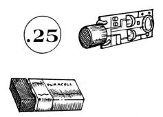
*Two commercially available wireless listening devices;* the top one can be wired to a battery or electrical source in the residence/vehicle. The bottom one is connected to a 9V battery.
