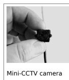
For surveillance operations. miniature CCTV video cameras are also routinely used. They have filmed people making and selling drugs, weapons, & bombs, as well as making incriminating statements. Mini-CCTV cameras can be as small as a dime in diameter (with a small pin-hole aperture). Like listening devices, mini-video cameras can be hidden in almost anything, inc. a pager, a teddy bear,
